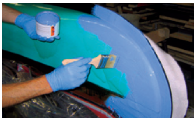
Application of the surface layer
