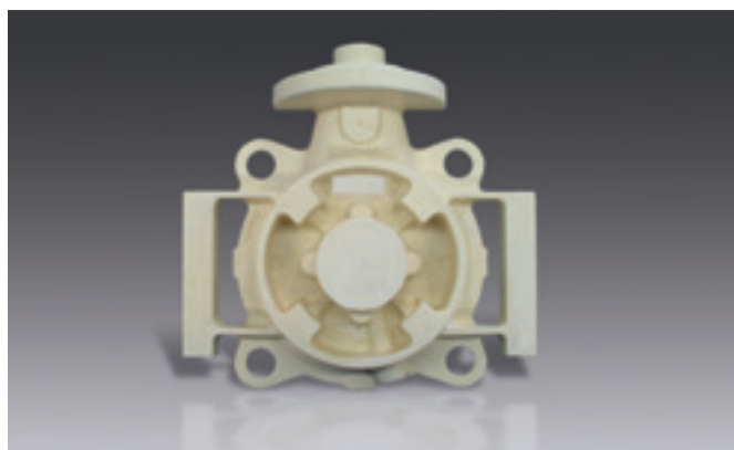
Pattern made of SG 700
