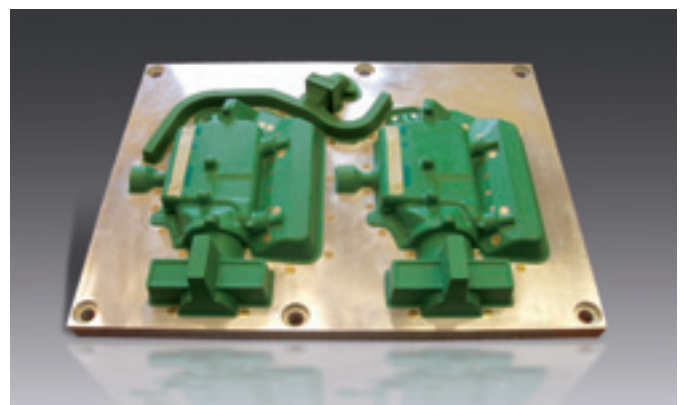
Pattern made of ebaboard PW 920
